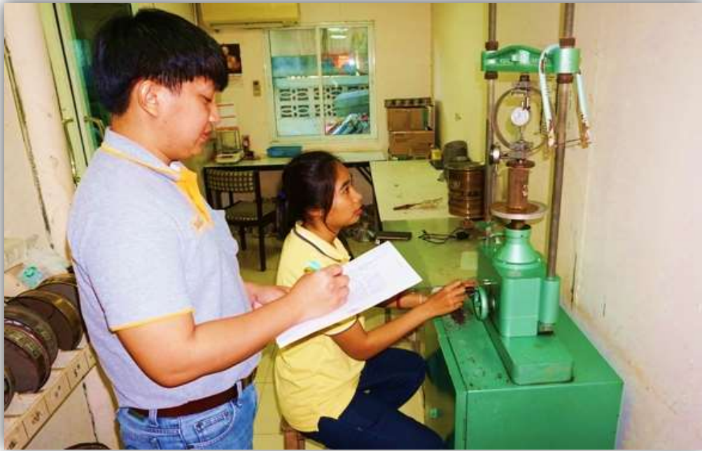
Unconfined Compression Test
